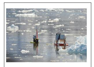
Figure 2: The multisampler (right) towed by an Unmanned Semi-Submersible Vehicle (USSV; left).
