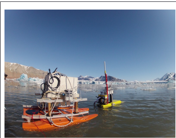
Figure 1: Shark unmanned semi-submersible vehicle and the automatic water multisampler in proximity of the Kronebreen glacier
