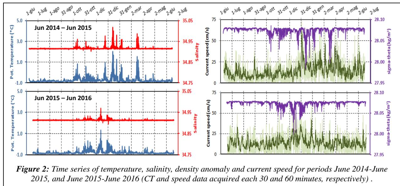
Figure 2: Time series of temperature, salinity, density anomaly and current speed for periods June 2014-June 2015, and June 2015-June 2016 (CT and speed data acquired each 30 and 60 minutes, respectively).
