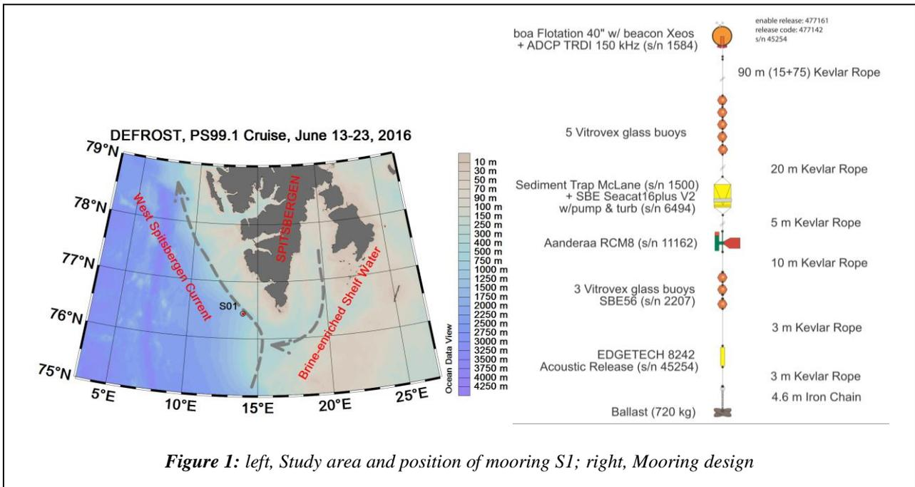
Figure 1: left, Study area and position of mooring S1; right, Mooring design
