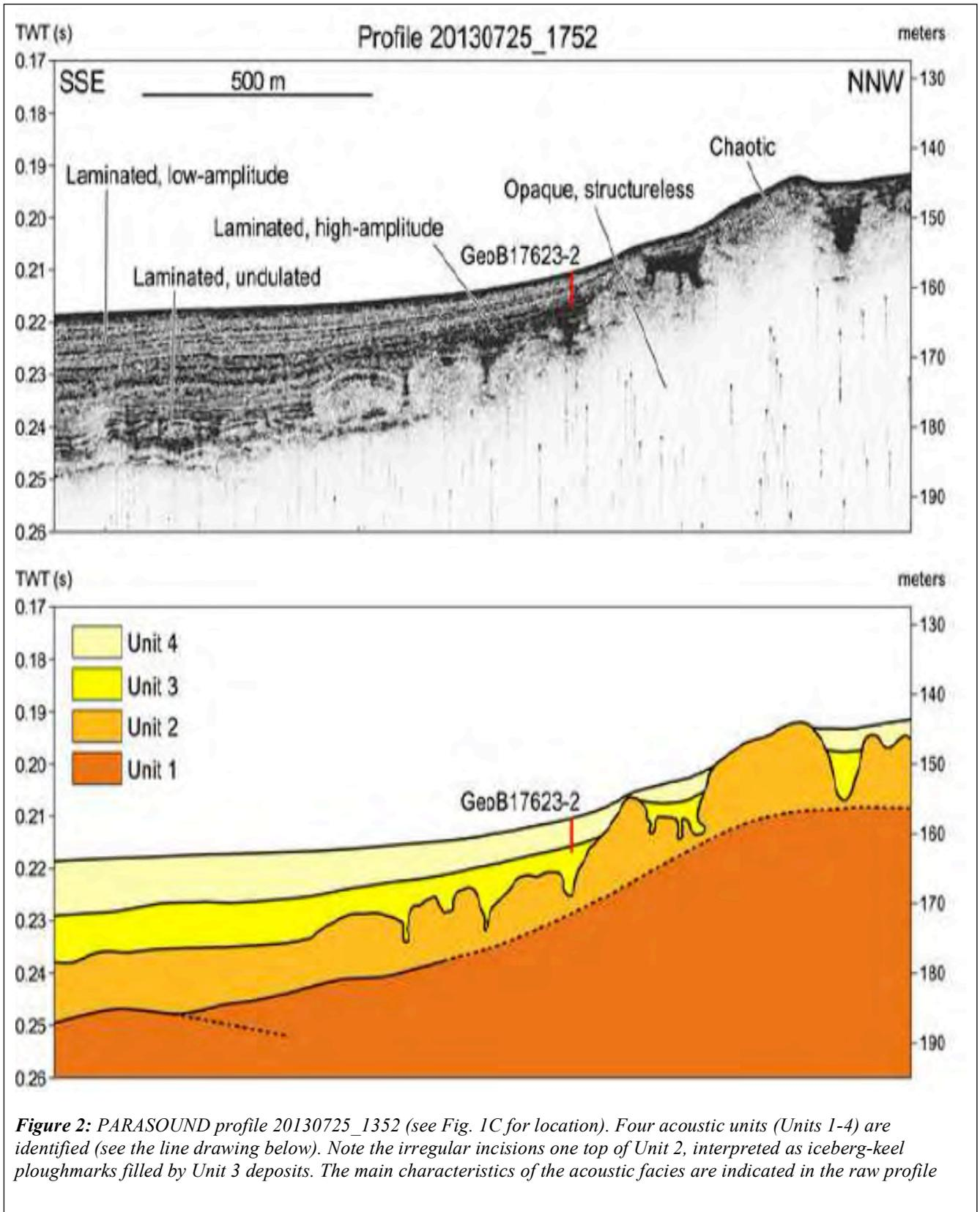
**Figure 2:** PARASOUND profile 20130725\_1352 (see Fig. 1C for location). Four acoustic units (Units 1-4) are identified (see the line drawing below). Note the irregular incisions one top of Unit 2, interpreted as iceberg-keel ploughmarks filled by Unit 3 deposits. The main characteristics of the acoustic facies are indicated in the raw profile
